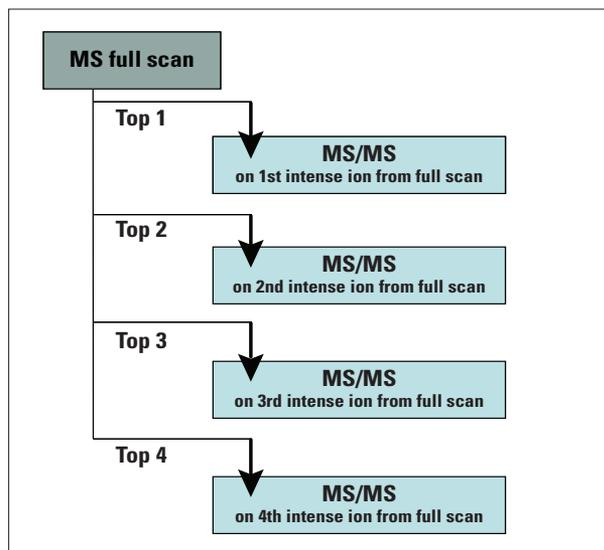
Figure 1: A schematic of the MS experiment
